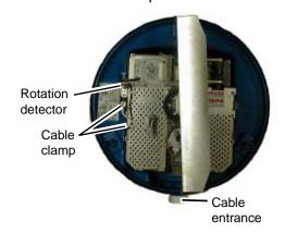
Antenna unit, cover removed, top view
