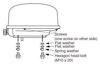
Antenna unit, showing location of mounting hardware
