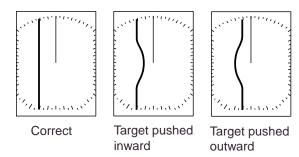
Improper and correct sweep timing
