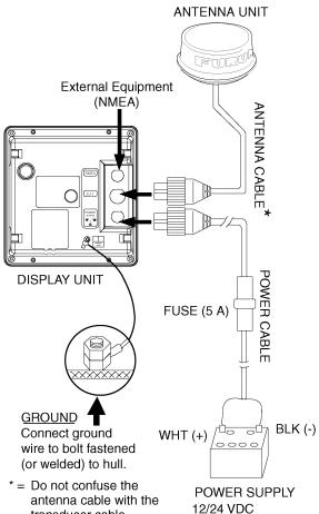
transducer cable for the Echo Sounder LS-6100. The transducer cable is black; the antenna cable is white and "RADAR" is written on the cable.
